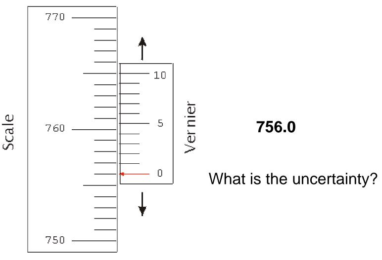
Smallest measurement on the main scale- Smallest measurement on the Vernier
