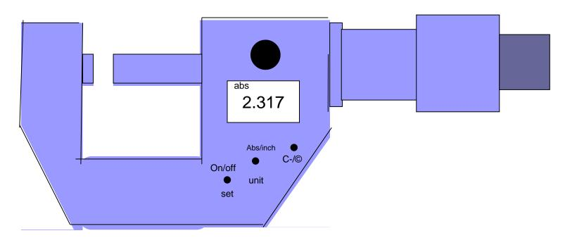
Using **only the ratchet** close the caliper.
